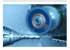
+ Low grinding forces: The combination of process optimised diamond quality, the new metal bond system and innovative production technology guarantee low grinding forces.
