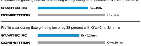
Kr ... Edge radius measured after grinding
