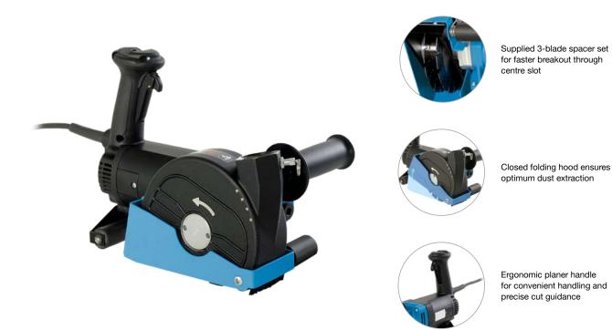
The HCE150 wall chaser is the ideal machine for cutting grooves and ducts in concrete, sand-lime brick or masonry. The slot width can be adjusted in 1 mm steps in the range 7-46 mm and the depth of cut can be continuously adjusted up to 45 mm. The supplied 3-blade spacer set permits faster breakout through
