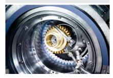
System solution: The design and specification of MIRA REX honing wheels are perfectly tailored for use with MIRA DDG diamond dressing gears.
