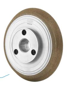
+ Maximum lifetimes: A galvanic bond matrix with exceptionally high bond strength keeps the application-specific grain in the bond, even during demanding machining processes. Owing to the special manufacturing process, superabrasives are distributed evenly across the profile and ensure maximum profile retention.
