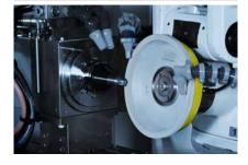
+ Better cutting ability: The bond system is characterised by a higher porosity at the same effective hardness of the grinding tool. This allows greater grinding power to be achieved.
